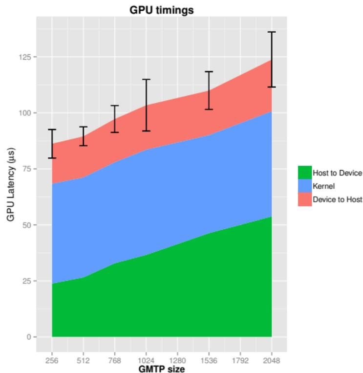
Preliminary latency tests performed with a **single-ring fitting** kernel.
